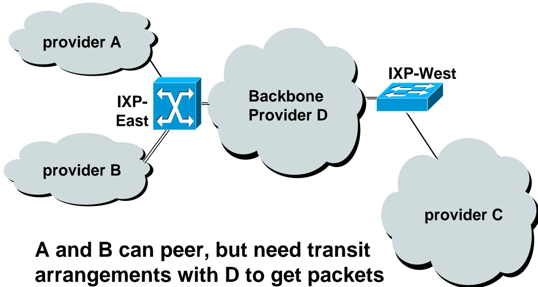
**A and B can peer, but need transit arrangements with D to get packets to/from C**
