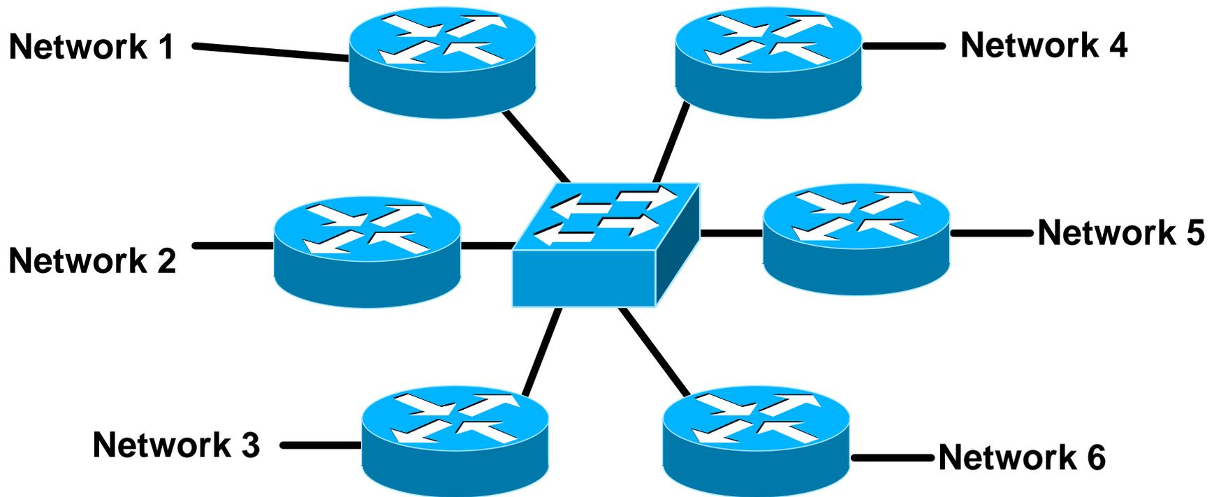
each of these represents a border router in a different autonomous system
