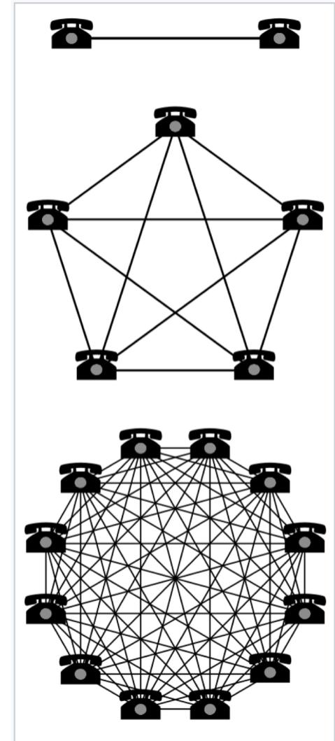
Two telephones can make only one connection, five can make 10 connections, and twelve can make 66 connections.
