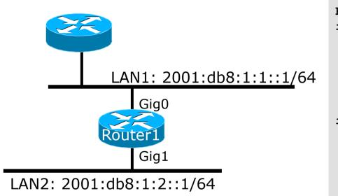
Dual stack IPv4/IPv6 multitopology configuration.
