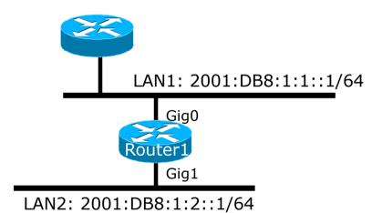
Dual stack IPv4/IPv6 multitopology configuration.
