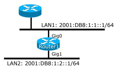
Dual stack IPv4/IPv6 single topology configuration.
