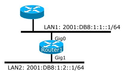
Dual stack IPv4/IPv6 single topology configuration.
