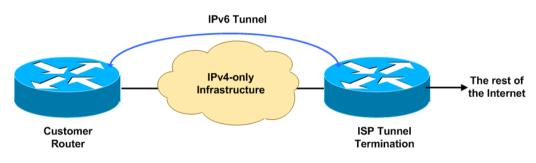
Figure 2 – IPv6 in IPv4 Tunnel
