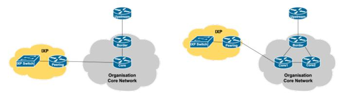
In more sophisticated cases, especially where the IXP is providing a significant portion of the organisation's traffic, a second peering router might be procured, to provide not only link redundancy but also router redundancy. This second/redundant infrastructure will likely only be deployed a bit further down the track, after gaining sufficient operational experience of traffic levels and infrastructure reliability. The digram below shows this scenario:
