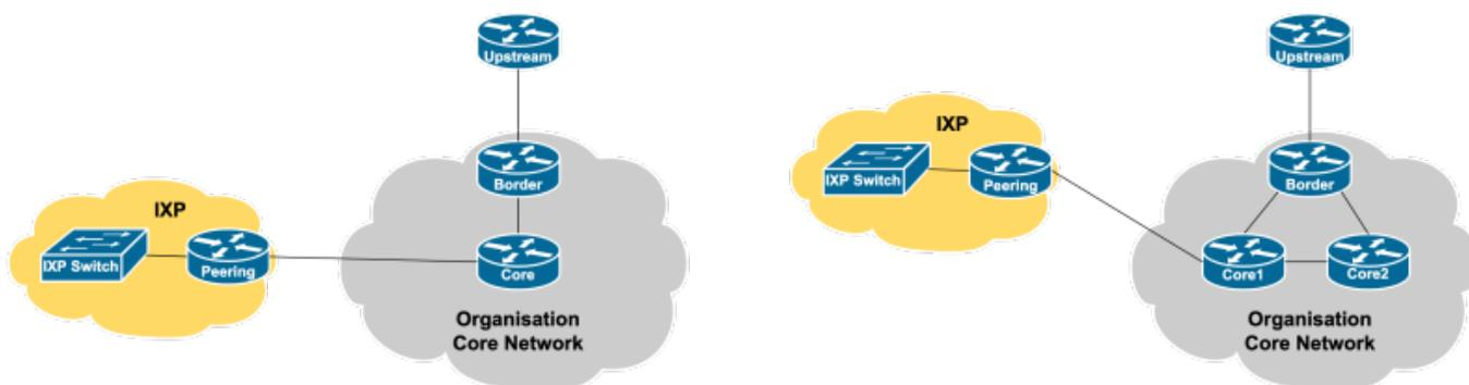
In more sophisticated cases, especially where the IXP is providing a significant portion of the organisation's traffic, a second peering router might be procured, to provide not only link redundancy but also router redundancy. This second/redundant infrastructure will likely only be deployed a bit further down the track, after gaining sufficient operational experience of traffic levels and infrastructure reliability. The digram below shows this scenario:
