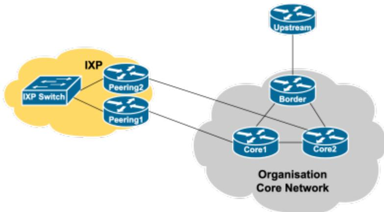
In the case the operator has private peers as well, these could connect to the peering router at the IXP (the Private Network Interconnect or PNI described elsewhere). Or, the operator would have a separate on-premises peering router.
