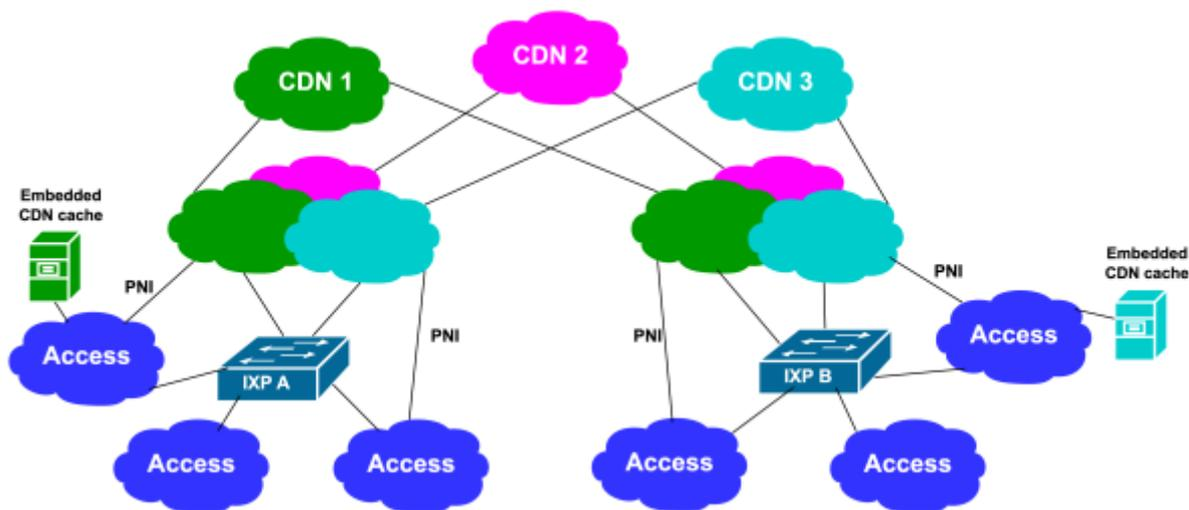
In the diagram, one Access Provider at IXP A hosts an embedded cache from CDN 1, and an Access Provider at IXP B hosts an embedded cache from CDN 3. Two other Access Providers only have a PNI with CDNs at the IXPs (no embedded cache server), and the other two Access Providers simply peer across the IX fabric (no PNI and no embedded cache server).
