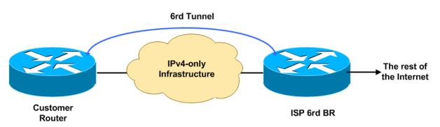
The Customer Router in the diagram is our Customer Router in our network. And the ISP 6rd BR capability will be configured on our autonomous system's Border Router.
